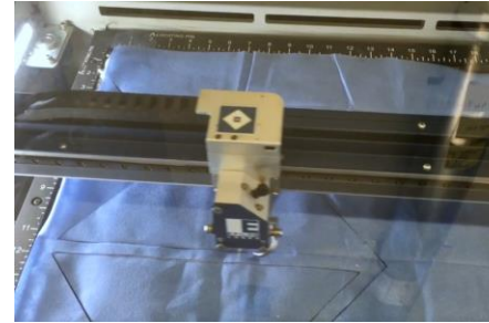
ARRANGE PATTERNS AND LASER CUT STACK. YOU SHOULD BE ABLE TO FIT 8 MASK PATTERNS PER MATERIAL STACK
