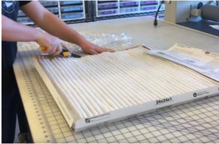
EXTRACT FILTER FROM FRAME (3L MASK ONLY, 2L MASK DOES NOT INCLUDE FILTER)
